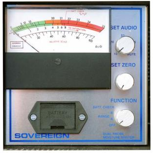
Nigel Clegg Associates - Yacht Coatings and Osmosis Specialists www.Passionforpaint.co.uk several weeks to dry. Similarly, epoxy coatings such as *International Gelshield Plus* and *Blakes GelProtect* can retain moisture for several weeks after lifting, and may result in high moisture readings during this time, (even if the laminate is perfectly dry underneath).
